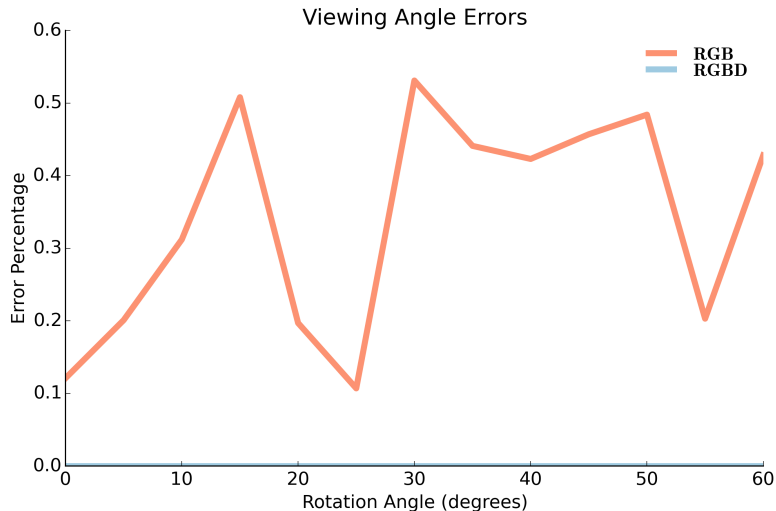
Figure 3.4: Viewing Angle vs Error Percentage (0.1 = 10%) under different simulated noise level. The new RGBD based algorithm can resist noise in the RGB image and it vastly outperforms the original algorithm.
